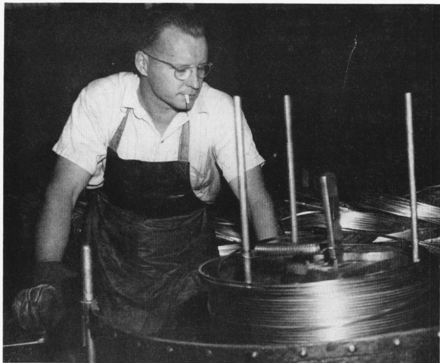
Absorbed in his work, John Nygard, a shaped wire drawer, is turning out a coil of wire on a drawing block in the Wire Mill. John has the ability to comprehend the difficulties of the problems involved in the work of drawing shaped wire. He is always on the lookout to make improvements.
